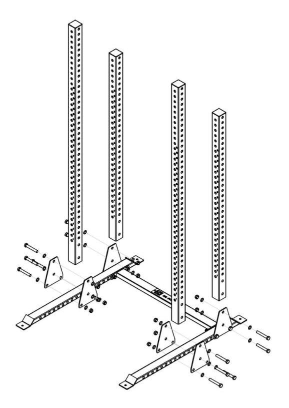
Attached the decline crossbeam (5) to upright (1&2), using M18x120 bolts(10).
