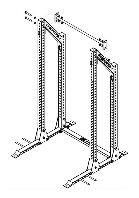
Insert the right and left sandwich J cup(8) into the proper postion of upright(1), also the band pins(9) to the base crossbeam(3).
