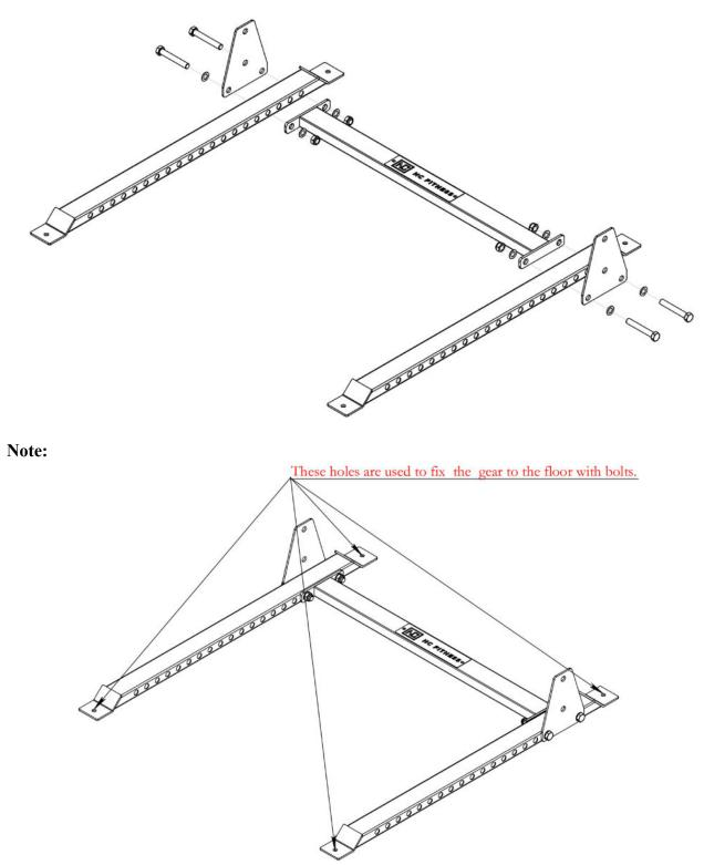
Attach the uprights (1&2) to the right base crossbeam(3) and the left base crossbeam(3) with connecting triangle plate(7), using M18x120 bolts(10).
